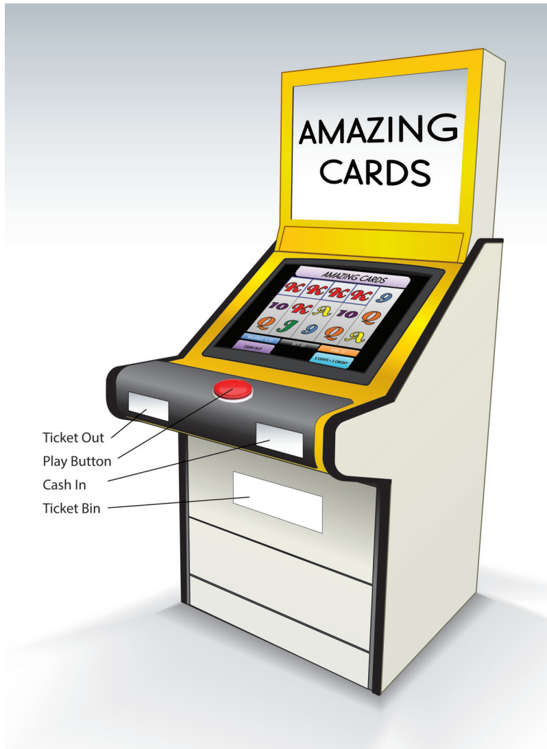
Figure 2. A schematic representation of a TapTix machine.
